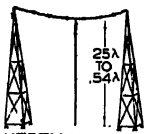
VERTICAL SINGLE-WIRE ANTENNA
